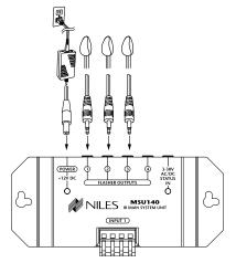
Figure 10: Connecting Power Supply and Flashers
